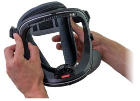
In case the visor has to be replaced or separately cleaned, it can be easily removed and attached back to the hood using two simple locking knobs. The face seal ensures secure and comfortable fit for the wearer. Thanks to a fast click-in system the face seal can be easily and quickly removed and attached back. The face seals can be washed in a washing machine and even dryed in the dryer. 4
