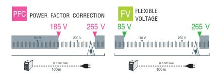
■ The latest generation of plasma 31FV is equipped with a PFC and Flexible Voltage With this technology, CUTTER 31FV works on either 110V(32A) or 230V(16A) or any voltage in the range of 85V-265V – combined with the PFC the cutting performance is maintained even during intensive use on power generator and when run with long extension leads (up to 100m).
