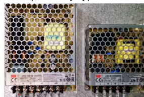
Double switching power supply
